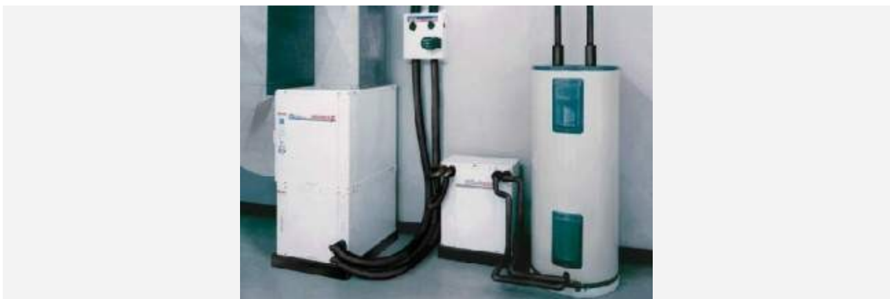
Ground source (a.k.a. geothermal) heat pumps, like the appliances above in combination with a long loop of tubing in the ground, use one half to one third the energy of conventional furnaces and air conditioning, generate domestic hot water, while running on electricity alone. While the appliance itself is not that expensive the digging or drilling of the ground loop makes the cost of the system substantially more than conventional units. As this represents a paradigm shift in heating and cooling, rebate programs by utilities or governments can help build a still small industry.
