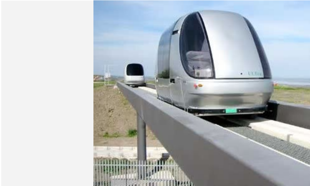
PRT advocates believe that people will prefer traveling in private pods routed automatically to their selected destination station on the PRT network
